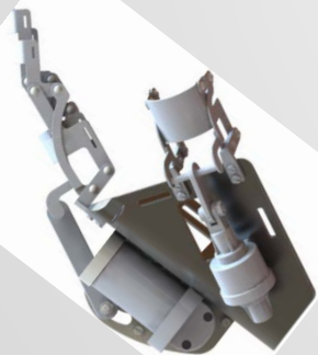
Wearable exoskeleton rehabilitation hand
