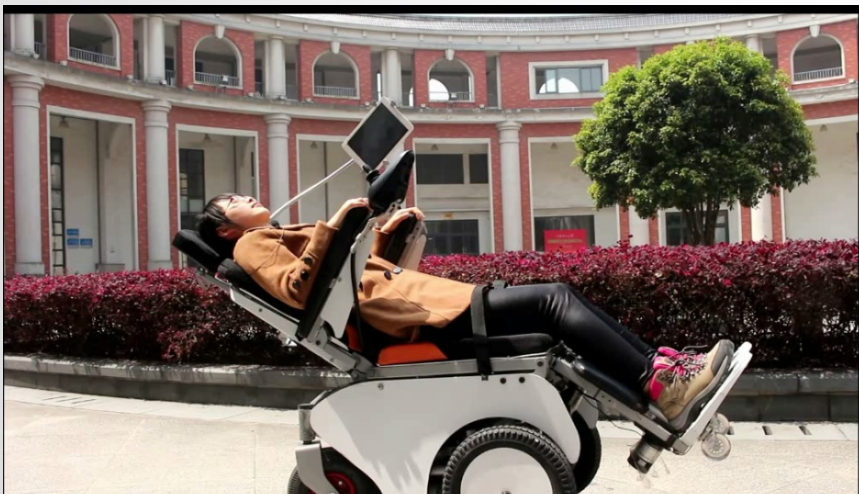
语音控制下肢被动训练 Voice control the lower limb passive training
